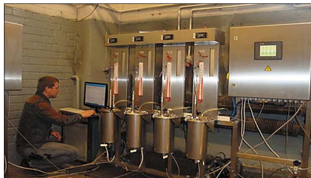
Fig. 2. A laboratory device consisting of four 5 l bioreactors
