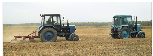
Fig. 3. Measuring plow traction resistance in field conditions
