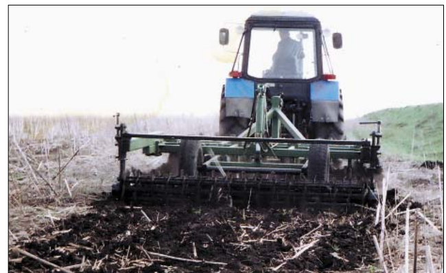
Fig. 5. RVK-4 cultivator-leveler operating on sunflower stubble
