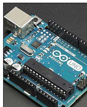
Fig. 3. Arduino Uno Board
