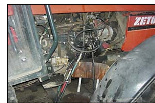
Fig. 2. System of connection of fuel box with flowmeter Macnaught M2ASP-1R to the fuel system of tested tractor ZETOR 10540
