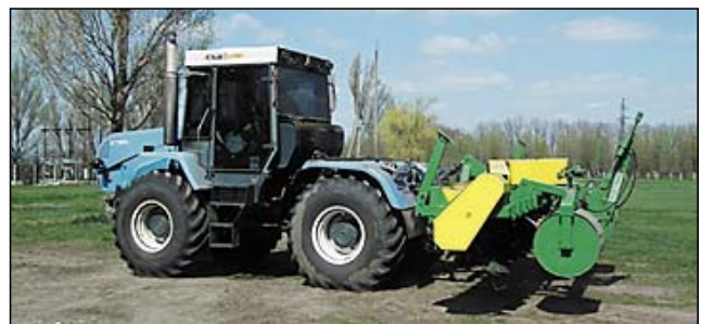
Fig. 1. The experimental soil-cultivating friable-separating machine aggregated with tractor XT3-17221
