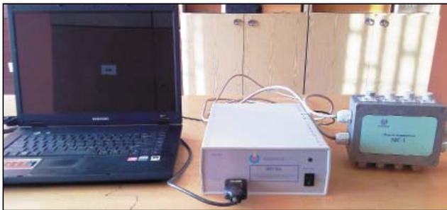
Fig. 1. General view of the testing system IP-264 connected to the laptop and the module of coordination MC-1
