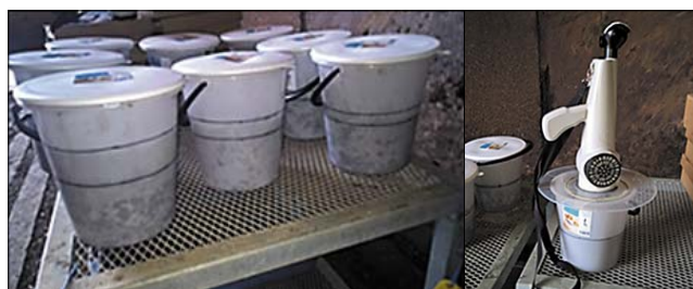
Fig. 2. Arrangement for the measurement; lids were used on the buckets between measurements (left), the olfactometer placed tightly on the bucket during measurement (right)
