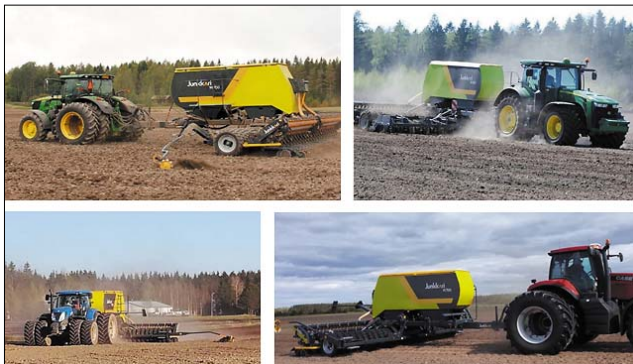
Fig. 5. User-Centred testing of the 7 m wide Junkkari W700™ combine drill for seed and fertilizer
