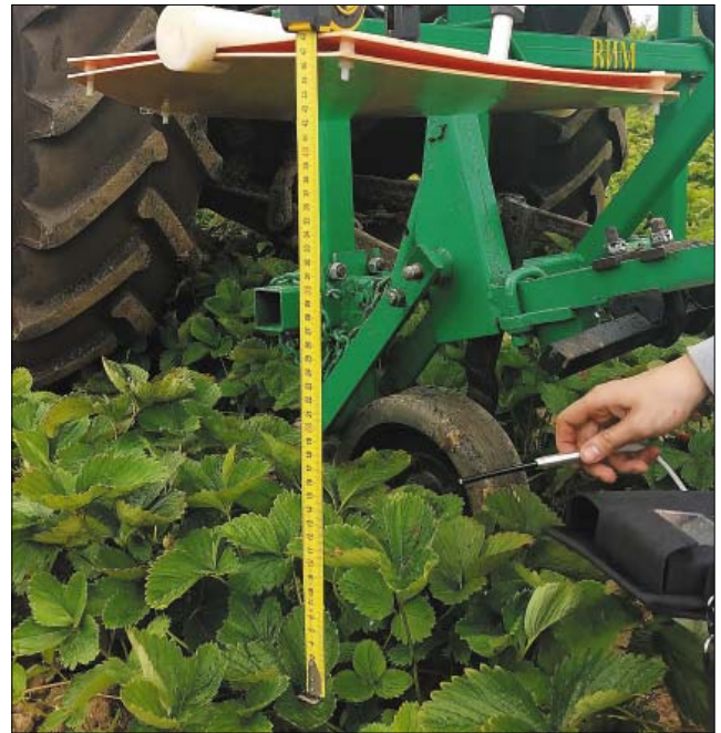
Fig. 2. Measuring distance from the working elements to the plant and the magnetic induction when performing the technological operation of MPT
