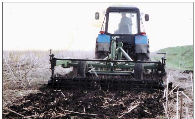
Fig. 5. RVK-4 cultivator-leveler operating on sunflower stubble
