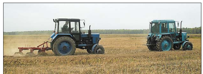
Fig. 3. Measuring plow traction resistance in field conditions
