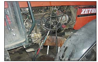
Fig. 2. System of connection of fuel box with flowmeter Macnaught M2ASP-1R to the fuel system of tested tractor ZETOR 10540
