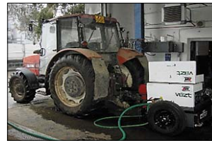
Fig. 1. Measurement with mobile dynamometer AW NEB 400 of external speed characteristics and consumption of tested fuels in tractor ZETOR 9540
